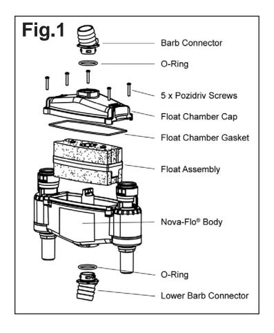
It is recommended that a bi-annual check is carried out to confirm correct functioning of the unit. If foreign matter is obstructing the movement of the float in the central chamber then cleaning will be required but access to the chamber is very simple. In most cases maintenance can be performed without needing to remove the unit from the bath.
